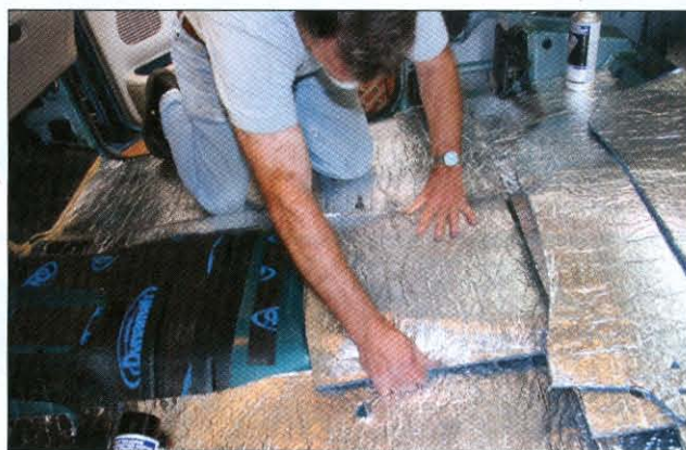
After adhesive is applied to both surfaces, put the Quality Heat shield on the Dynamat strips.
